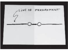
exposure of a uniform PMMA block. Always measure the optical density differences in a line perpendicular to the tube axis to avoid influence of the heel effect.
